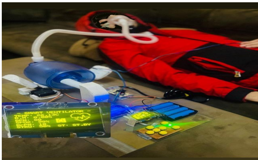
Figure 6. Practical experimental setup of the proposed ventilator system during testing.
