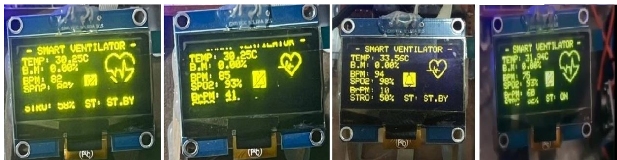
Figure 7. Real-time physiological measurements displayed on the OLED screen.
