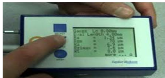
Figure 3: Roughness test device (Surtronic 25).
